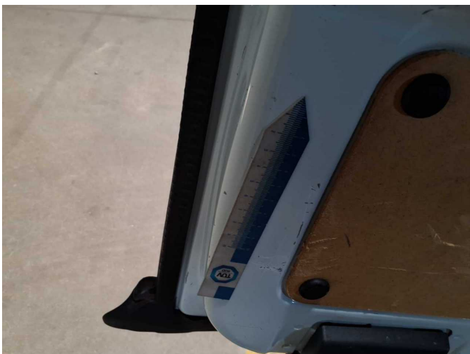
Damage 6: Boot lid / rear door: Rear door - left side - Dent / paintcoat damage - Repair and paint
