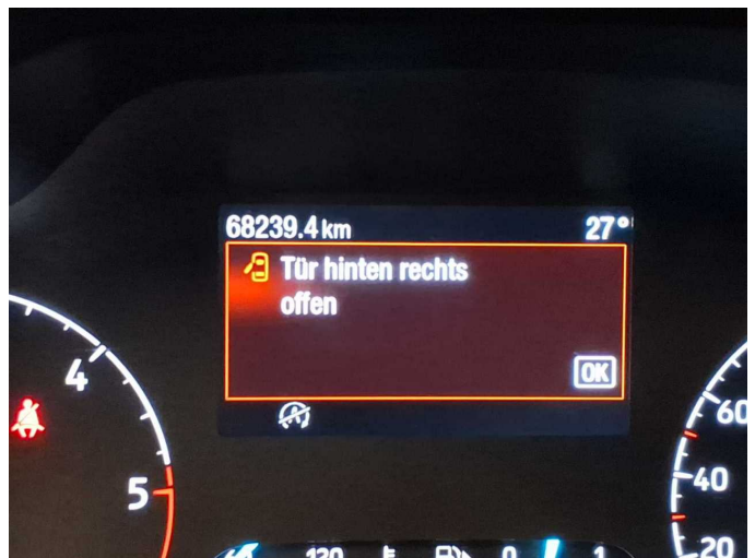
Damage 1: Instrument panel: Indicator light (Meldung Tür offen obwohl Tür zu) - Electrical fault - Perform diagnosis
