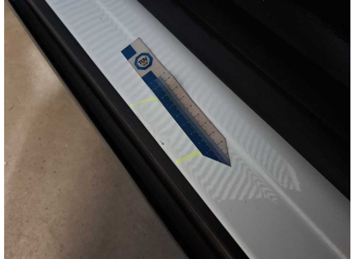
Damage 5: Sill - left side: Sill - Dent / paintcoat damage - Repair and paint
