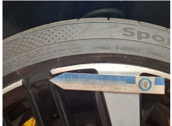
Damage 11: Wheel / tyres: Alloy rim - front left side (Materialabtrag) - Scratched - Replace
