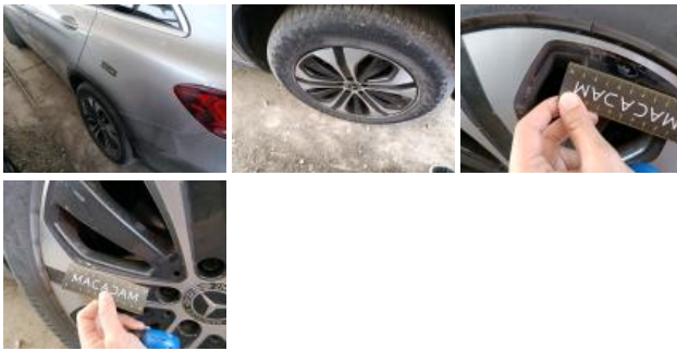
Tyre RR, Out of tolerance, Replace
