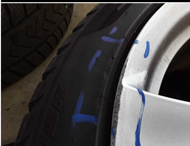
Damage #2: 2nd wheel set: Tyres - complete set - Worn - No deduction
