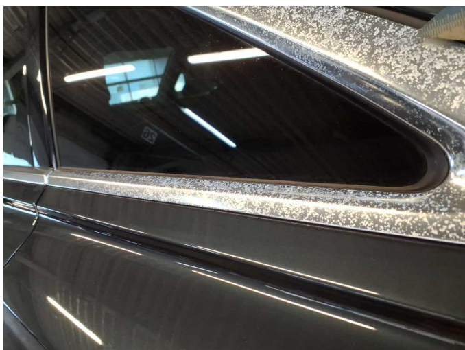
Damage 12: Trim / covers: Brightware / decorative strip (Dreieckfenster, Anätzungen) - Paint defect - Replace
