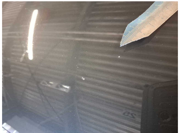
Damage 14: Bonnet: Bonnet - Stone chips - Paint
