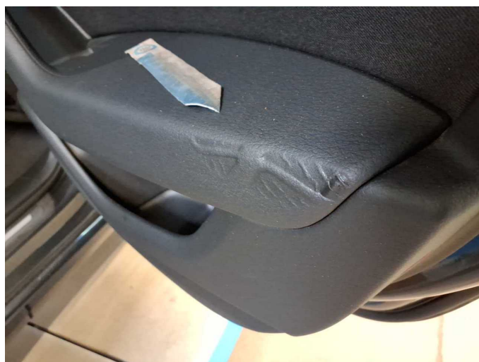
Damage 7: Door - rear right side: Door handle - inside - Deformed - Smart repair
