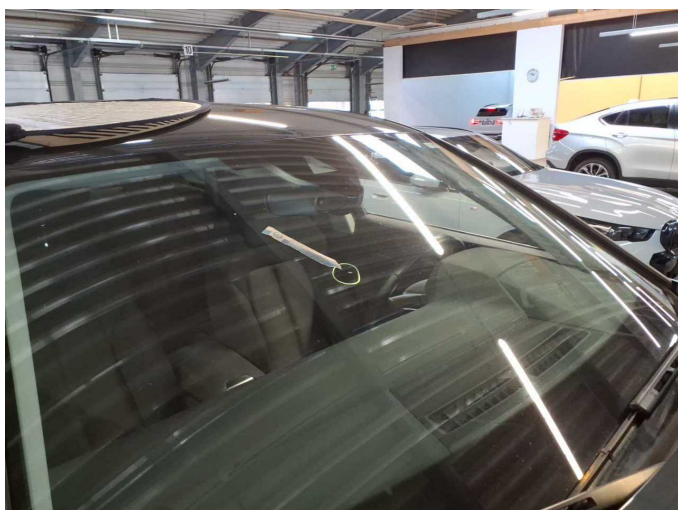
Damage 15: Vehicle glazing: Windscreen (Rissbildung) - Stone chips - Replace
