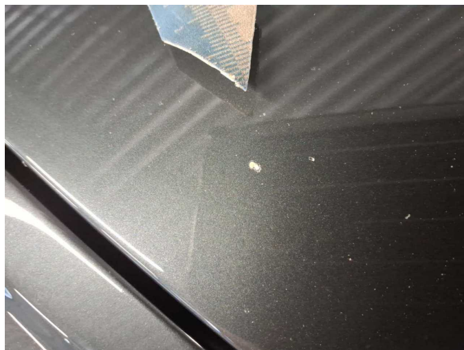
Damage 14: Bonnet: Bonnet - Stone chips - Paint
