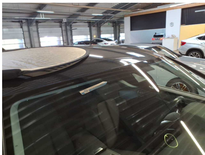
Damage 15: Vehicle glazing: Windscreen (Rissbildung) - Stone chips - Replace
