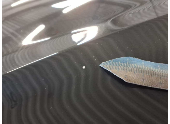
Damage 14: Bonnet: Bonnet - Stone chips - Paint
