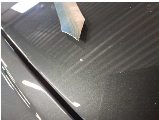
Damage 14: Bonnet: Bonnet - Stone chips - Paint
