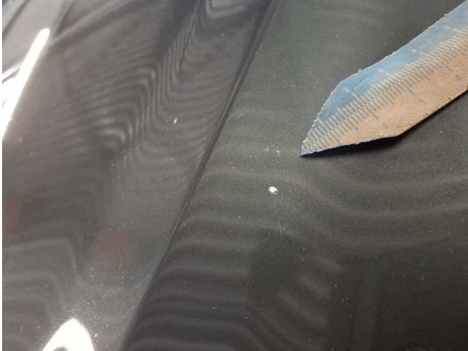
Damage 14: Bonnet: Bonnet - Stone chips - Paint
