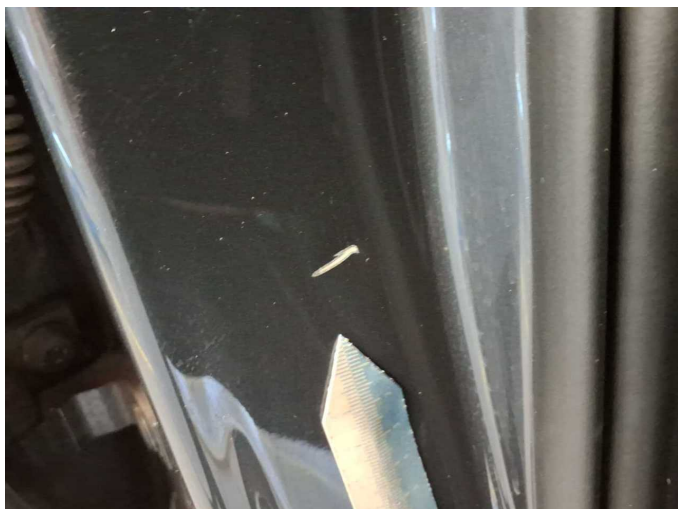
Damage 5: Body: B-pillar - right side - Dent / paintcoat damage - Smart repair
