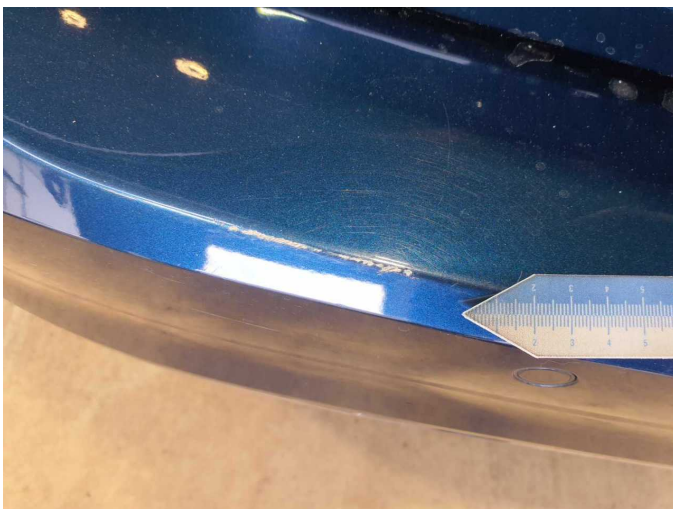
Damage 10: Rear bumper: Rear bumper - Scratch(es) - Paint
