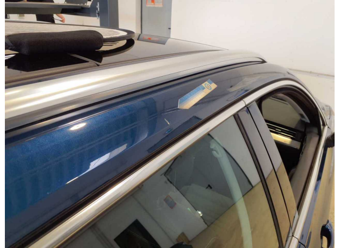
Damage 9: Roof: Roof rail - right side (Anätzung) - Paint defect - Repair and paint
