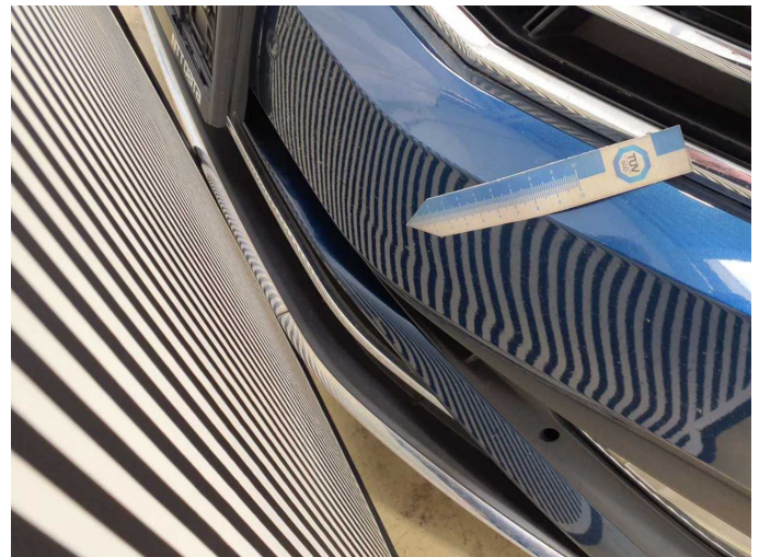
Damage 7: Front bumper: Front bumper - Dent / paintcoat damage - Loss in value
