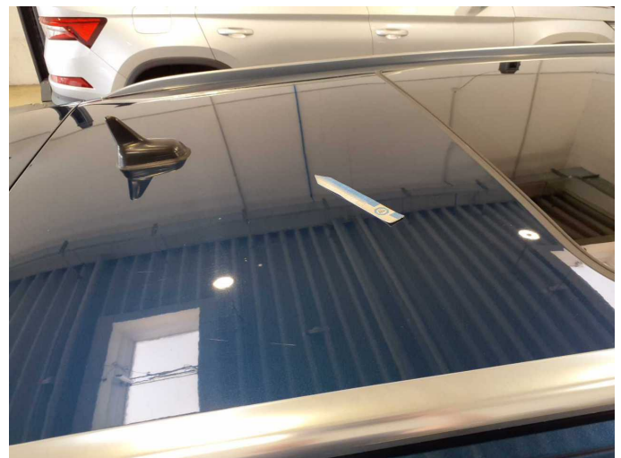
Damage 1: Roof: Roof - dent(s) - Smooth repair work
