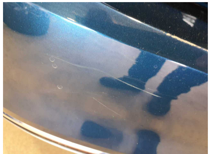
Damage 10: Rear bumper: Rear bumper - Scratch(es) - Paint
