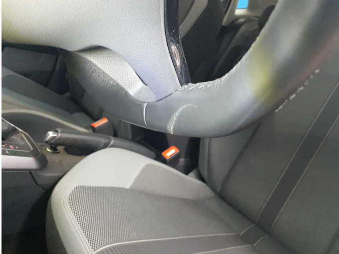
Damage 3: Steering system: Steering wheel - Scratch(es) - Smart repair
