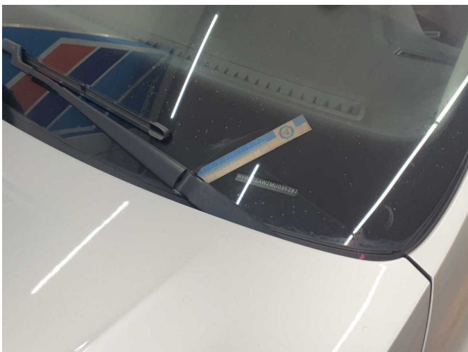
Damage 5: Vehicle glazing: Windscreen - Scratch(es) - Replace
