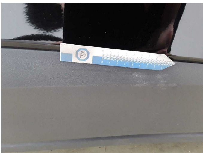
Damage 3: Door - front right side: Brightware - lower - Scratch(es) - Replace
