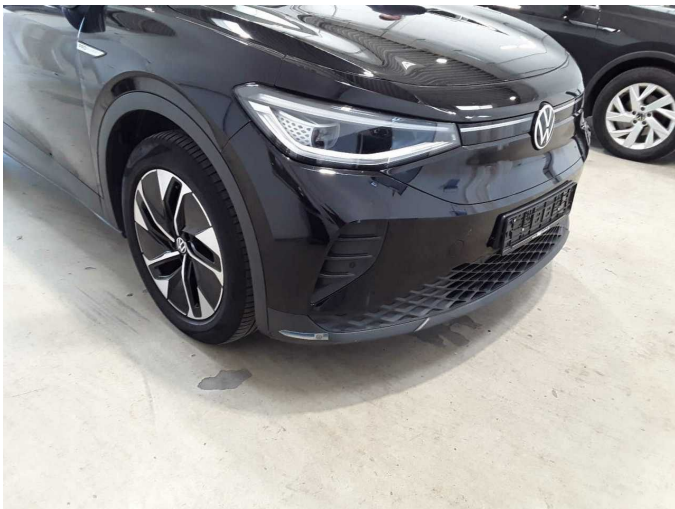
Damage 6: Front bumper: Spoiler - Scratched - Replace
