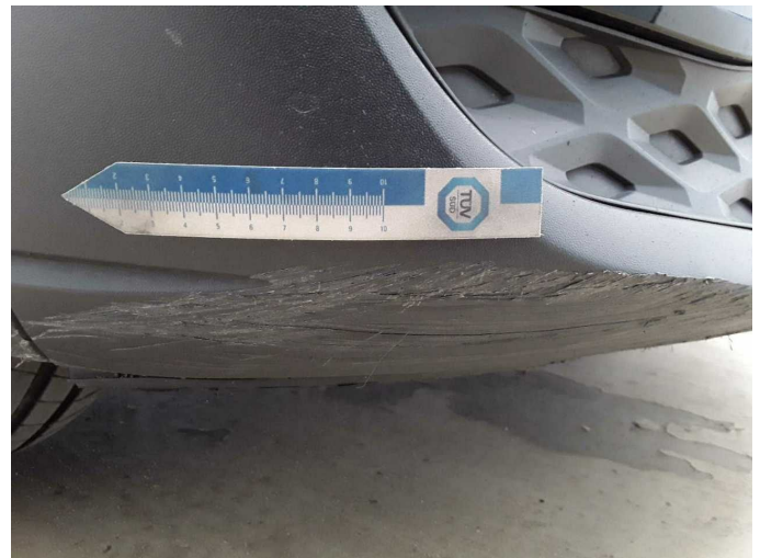
Damage 6: Front bumper: Spoiler - Scratched - Replace
