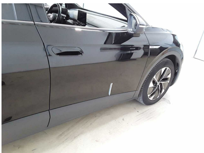
Damage 10: Door - front right side: Door - Deformed - Repair and paint
