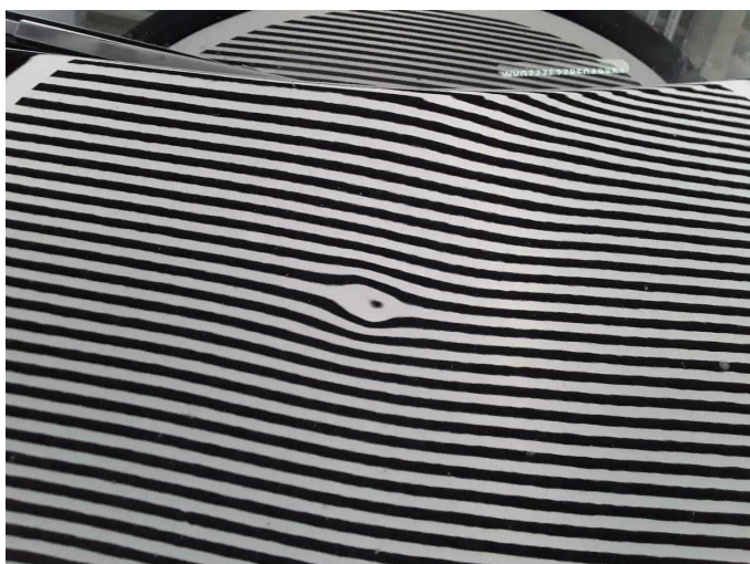
Damage 1: Bonnet: Bonnet - dent(s) - Smooth repair work
