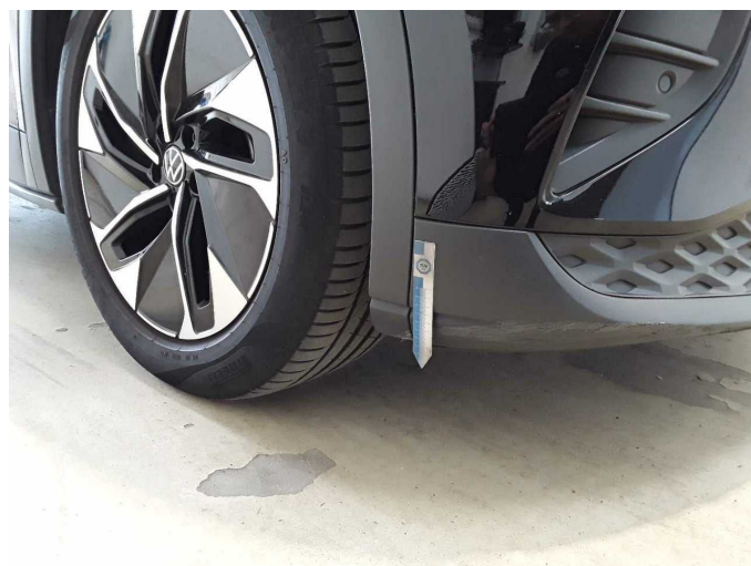
Damage 4: Mudguard - right side: Wheel well extension - Scratch(es) - Replace
