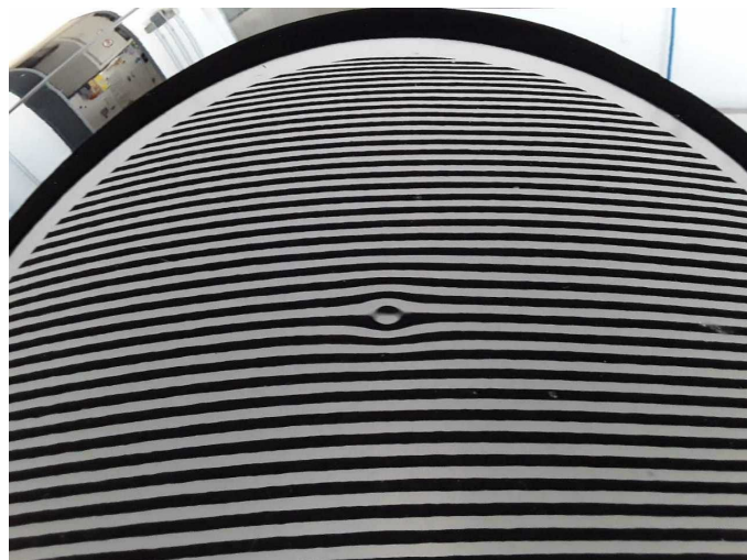
Damage 1: Bonnet: Bonnet - dent(s) - Smooth repair work
