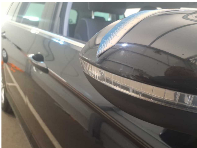
Damage 3: Indicator - front: Indicator - front (Blinker Spiegel Rechts) - Scratched - Replace
