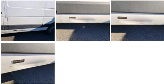
Outer sill R, Dent(s) and scratch(es), Replace and paint
