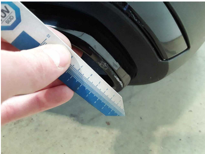
Damage 5: Rear bumper: Rear bumper (+ Blende ern+ becke Endrohr re ern.) - Scratch(es) - Paint
