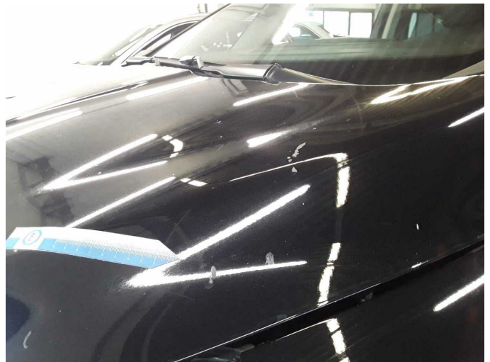
Damage 5: Bonnet: Bonnet (Harz) - Paint defect - Paint
