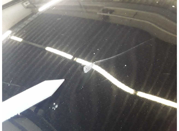
Damage 5: Bonnet: Bonnet (Harz) - Paint defect - Paint
