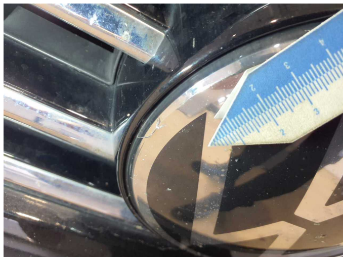
Damage 10: Front structure: Emblem - Broken / torn - Replace
