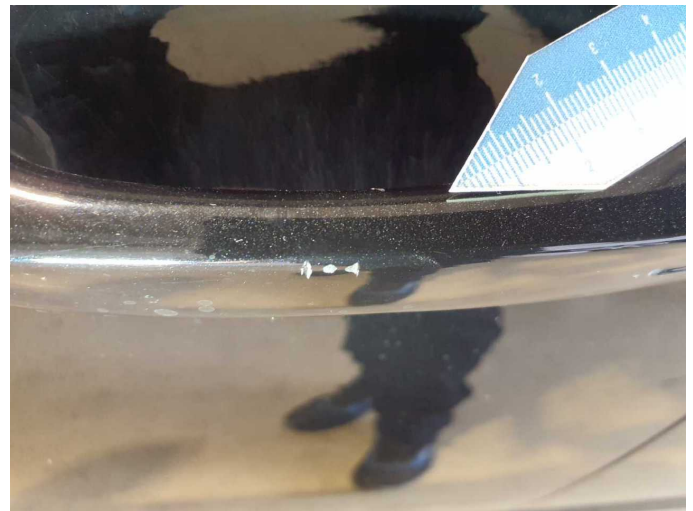
Damage 5: Door - front left side: Door handle - outside - Scratch(es) - Paint
