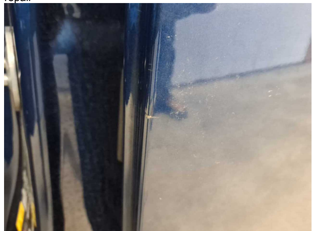
Damage 2: Door - rear left side: Door - Scratch(es) - Repair and paint
