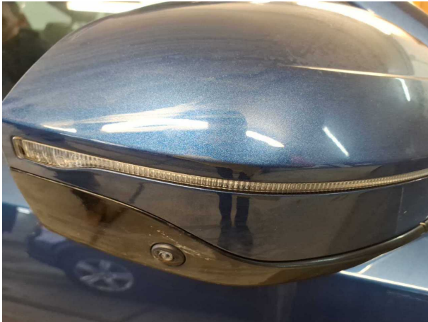
Damage 1: Wing mirror - right side: Cap - Scratched - Smart repair
