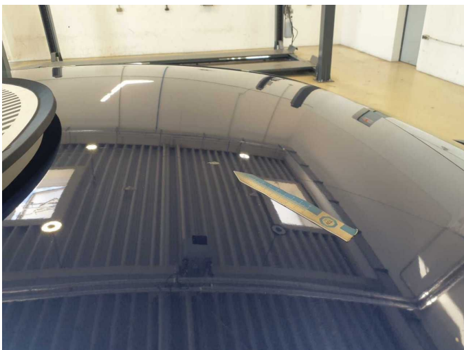
Damage 13: Roof: Roof (+Anätzung) - Dent / paintcoat damage - Repair and paint
