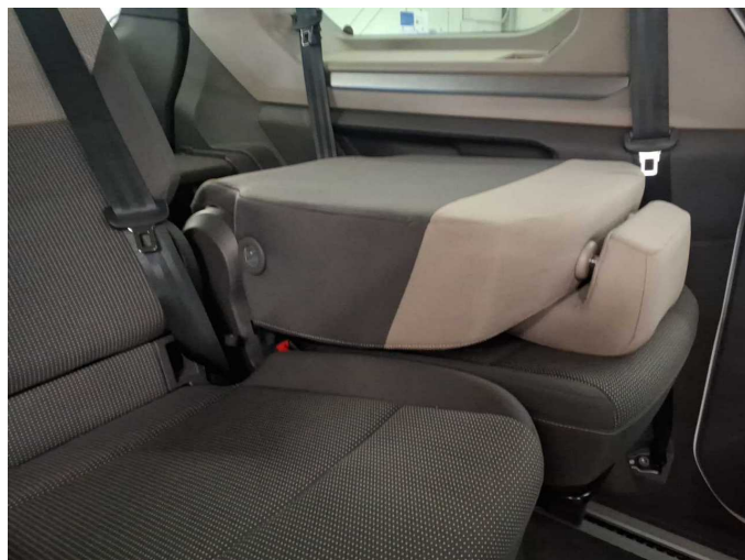
Damage 3: Seat - rear: Back seat (Sitzverstellung hinten Links klemmt) - Functional / admissibility - Perform diagnosis
