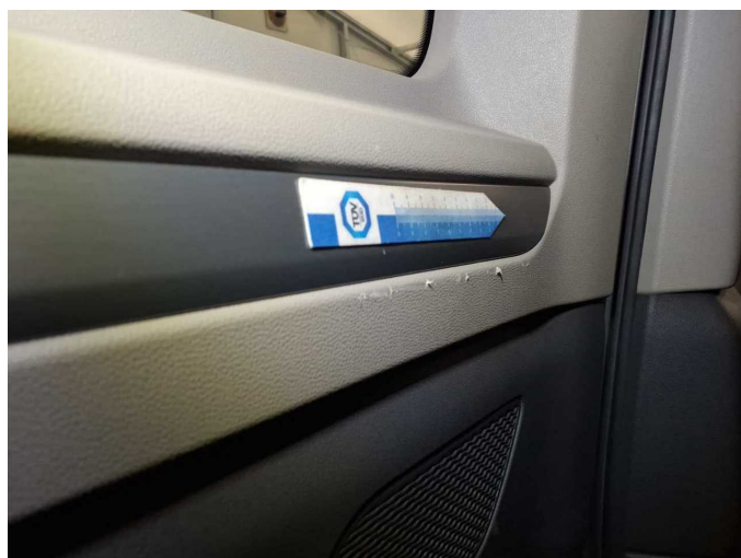
Damage 4: Trim / covers: Door trim - rear left side - Scratch(es) - Loss in value
