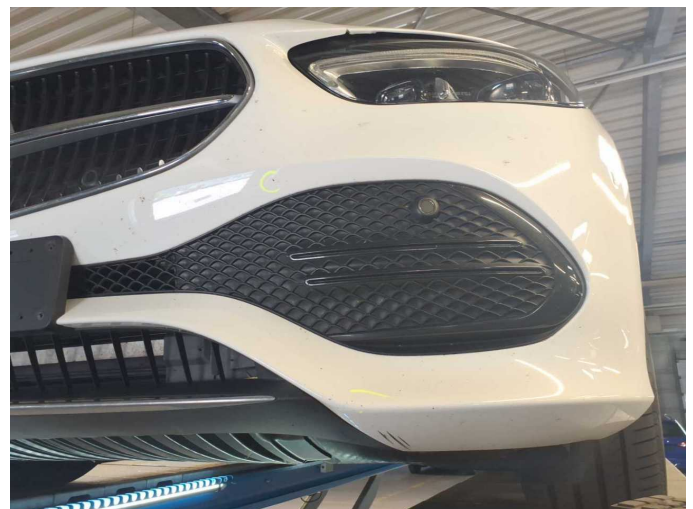
Damage 5: Front bumper: Front bumper - Scratch(es) - Paint
