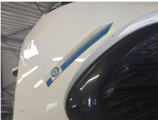
Damage 5: Front bumper: Front bumper - Scratch(es) - Paint
