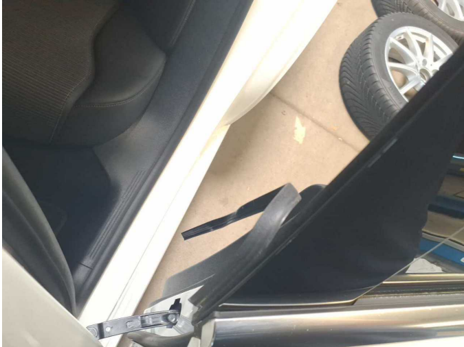
Damage 3: Door - rear left side: Door seal - Damaged - Replace
