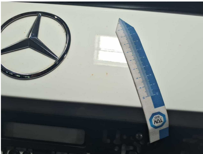
Damage 6: Boot lid / rear door: Boot lid (Rostpickel) - Corrosion - Paint
