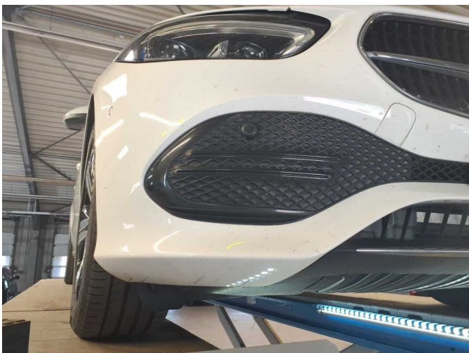
Damage 5: Front bumper: Front bumper - Scratch(es) - Paint
