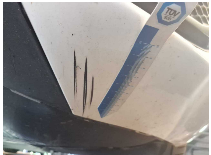
Damage 5: Front bumper: Front bumper - Scratch(es) - Paint
