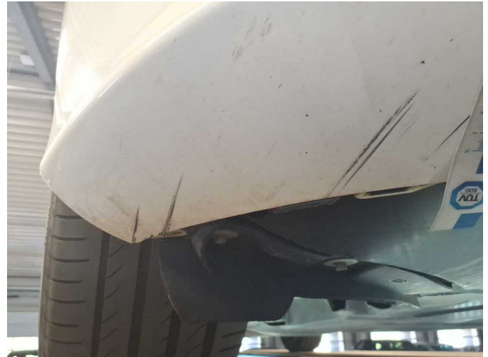
Damage 5: Front bumper: Front bumper - Scratch(es) - Paint
