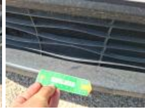
Bumper spoiler Rear, Deformed / Strained, Replace
