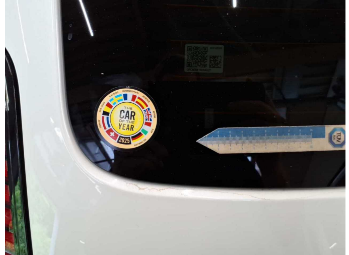
Damage 1: Vehicle glazing: Rear window - Glued / labelled - De-glug / neutralise
