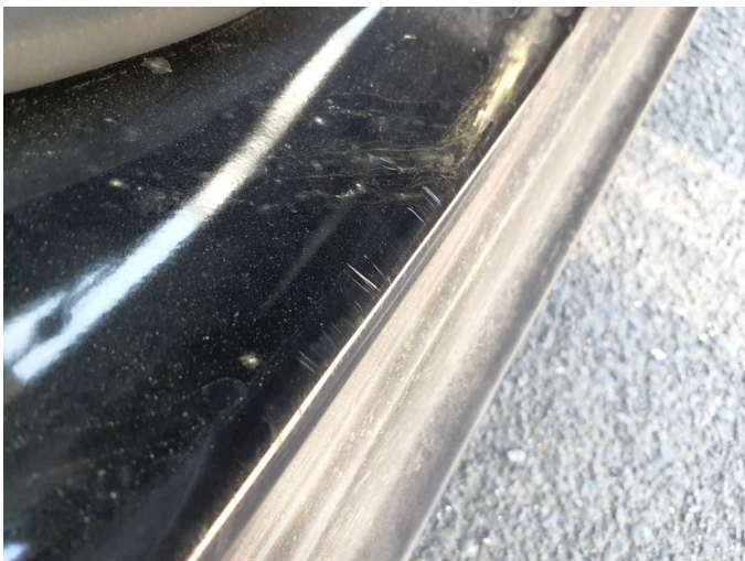
Damage 4: Sill - right side: Sill - Scratch(es) - Paint
