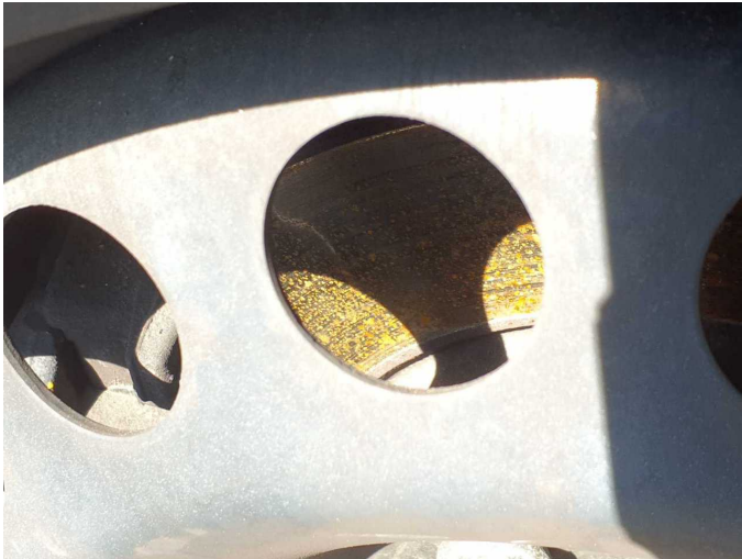
Wear and tear 2: Braking system: Brake discs and brake pads - front - Corrosion - No deduction
