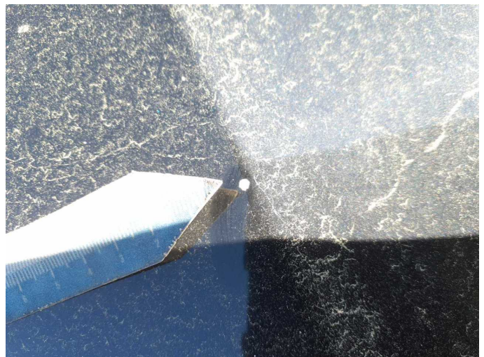
Damage 5: Bonnet: Bonnet - Stone chips - Paint
