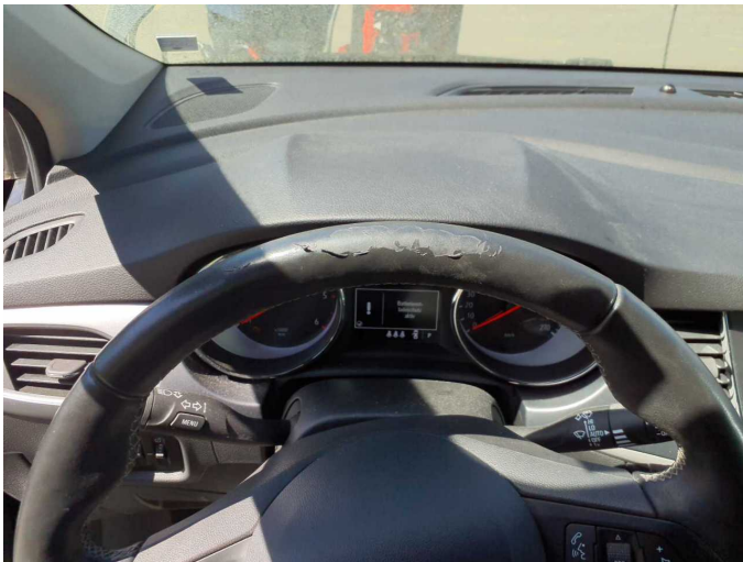
Damage 3: Steering system: Steering wheel - Scratched - Smart repair
