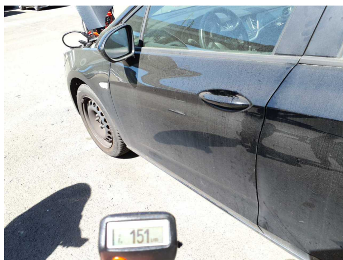
Repainting 4: Door - front left side
