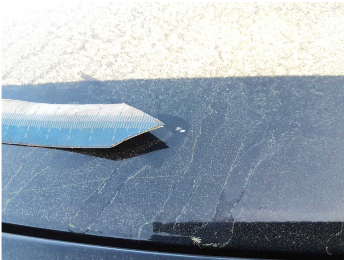
Damage 5: Bonnet: Bonnet - Stone chips - Paint
