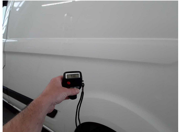
Side panel - rear left side: 198 \mu\text{m}
