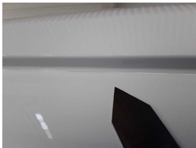
Damage 2: Side panel - rear right side: Side panel (Abklebekante) - Unprofessionally repaired - Paint
