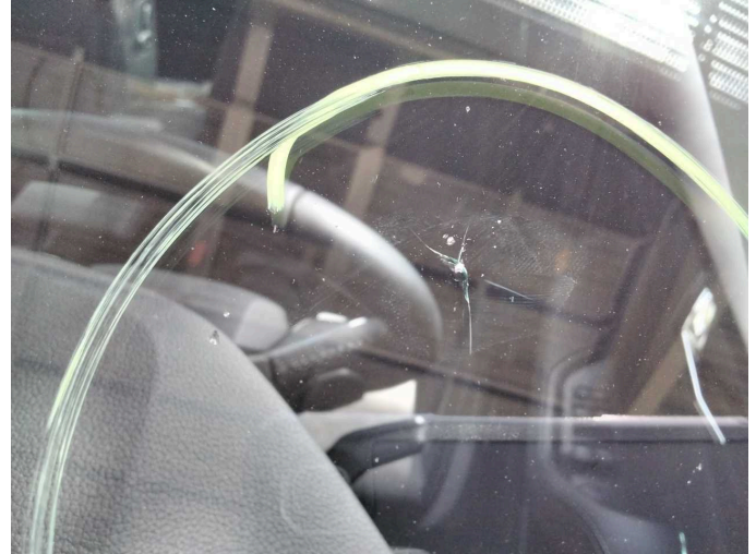
Damage 17: Vehicle glazing: Windscreen - Stone chips - Replace
