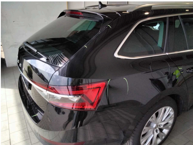
Damage 13: Side panel - rear right side: Side panel - Scratch(es) - Paint
