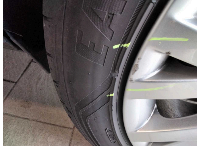
Damage 10: Wheel / tyres: Tyre - rear left side - Damaged - Replace
