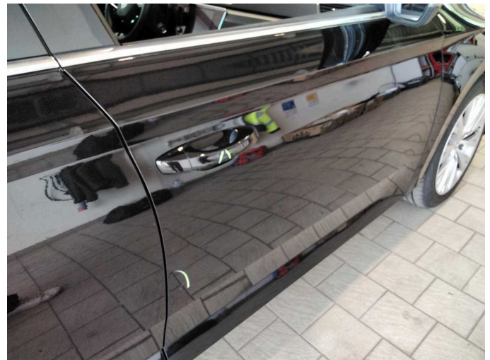
Damage 9: Door - front right side: Door handle - outside - Scratch(es) - Paint
