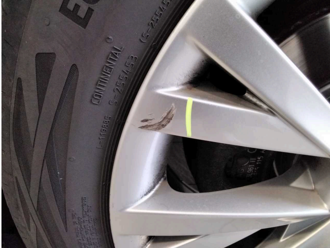
Damage 12: Wheel / tyres: Alloy rim - front left side - Scratch(es) - Loss in value
