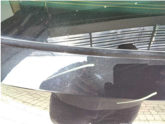
Damage 1: Boot lid / rear door: Boot lid - Scratch(es) - Smart repair
