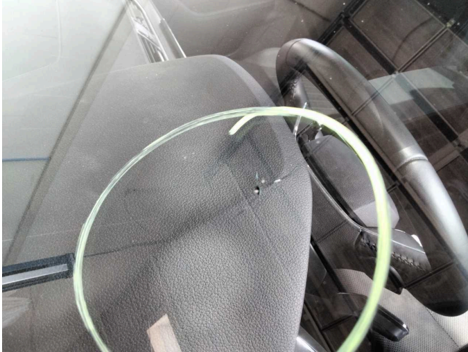
Damage 17: Vehicle glazing: Windscreen - Stone chips - Replace
