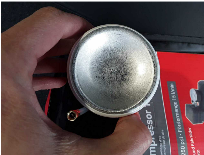
Wear and tear 4: Equipment: Tirefit filler - Expired - No deduction
