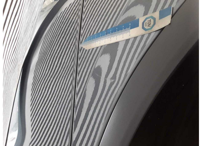
Damage 10: Mudguard - right side: Mudguard - right side - Dent / paintcoat damage - Repair and paint
