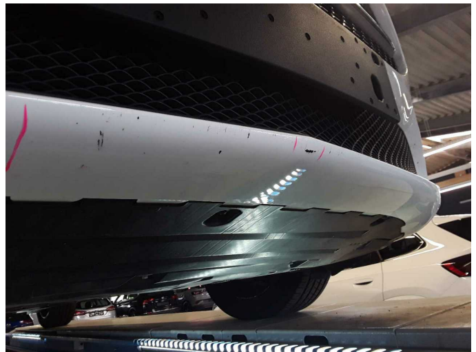
Damage 7: Front bumper: Front bumper - Scratch(es) - Paint
