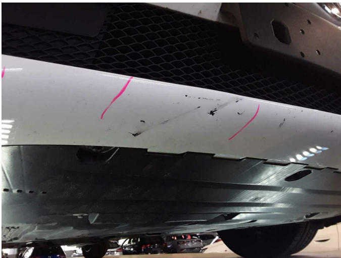
Damage 7: Front bumper: Front bumper - Scratch(es) - Paint
