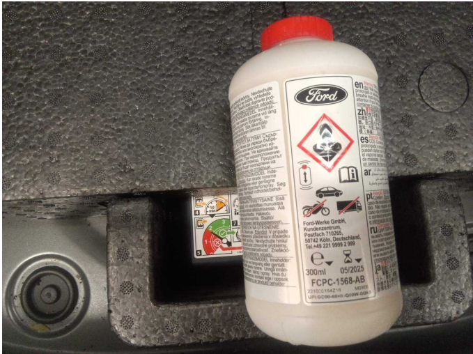
Damage 1: Equipment: Tirefit filler - Expired - Replace
