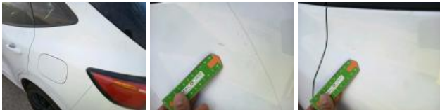
Door RL, Scratch(es), Repair and paint (complete)
