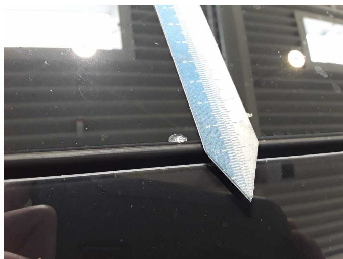
Damage 6: Roof: Sun roof / glass - Stone chips - repair according to calculation
