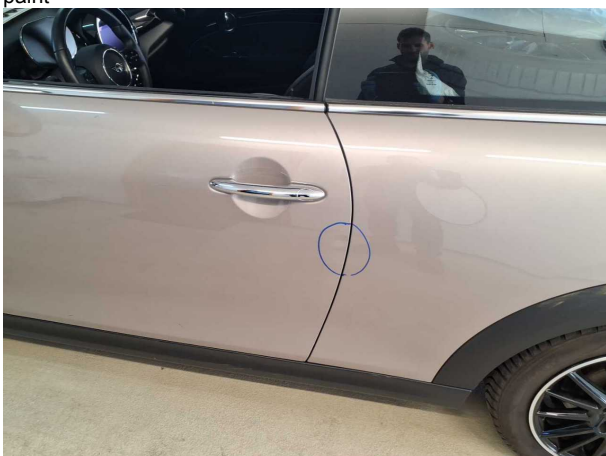
Damage #4: Door - front left side: Door - dent(s) - Repair and paint
