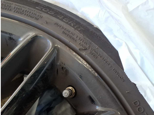
Damage #2: 2nd wheel set: 2 alloy rims - Scratched - Loss in value
