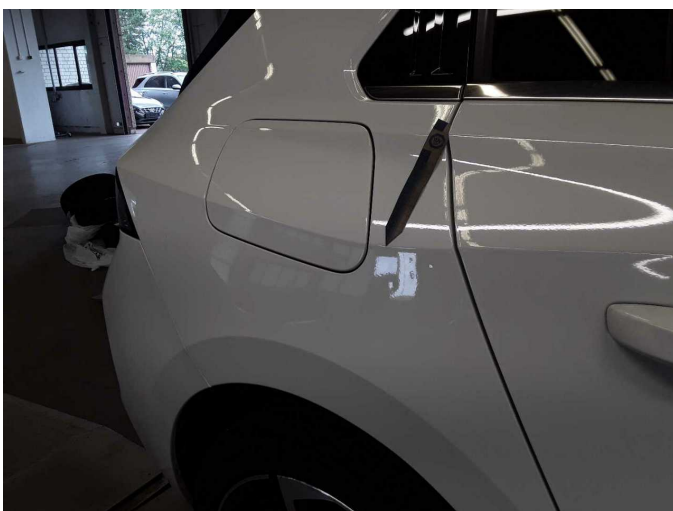
Damage 6: Side panel - rear right side: Side panel - dent(s) - Smooth repair work
