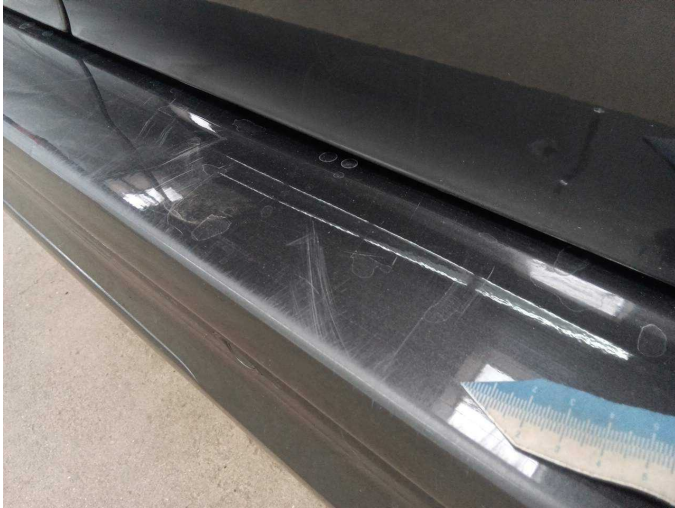
Damage 4: Rear bumper: Rear bumper - Scratch(es) - Paint
