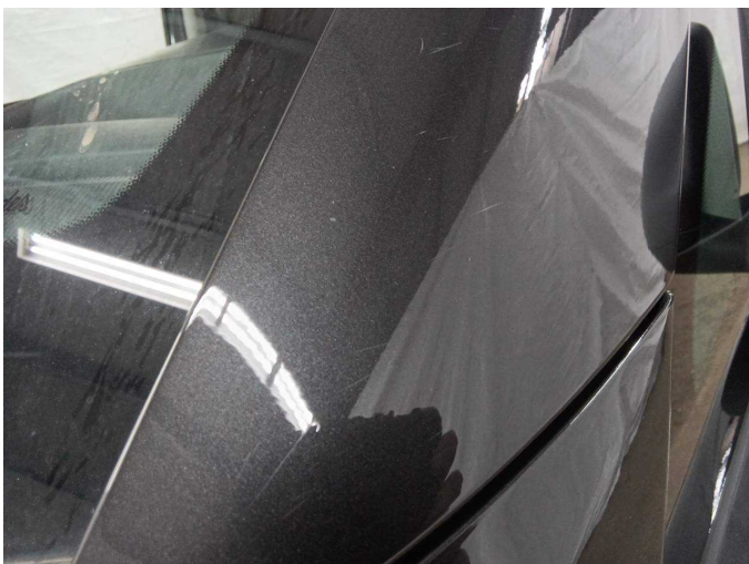
Damage 3: Body: A-pillar - left side - Scratch(es) - Paint
