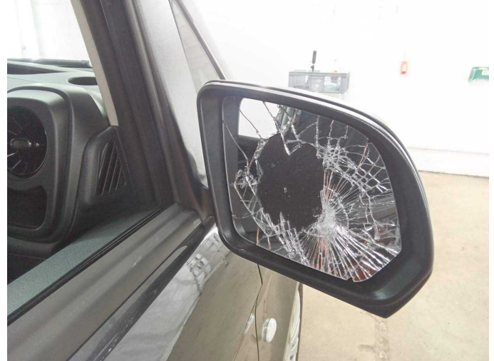
Damage 2: Wing mirror - right side: Mirror glass - Broken / torn - Replace
