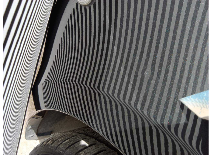
Damage 6: Mudguard - right side: Mudguard - right side - Dent / paintcoat damage - Repair and paint
