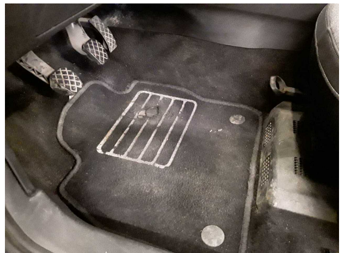
Damage 1: Trim / covers: Floor mats - Damaged - Replace
