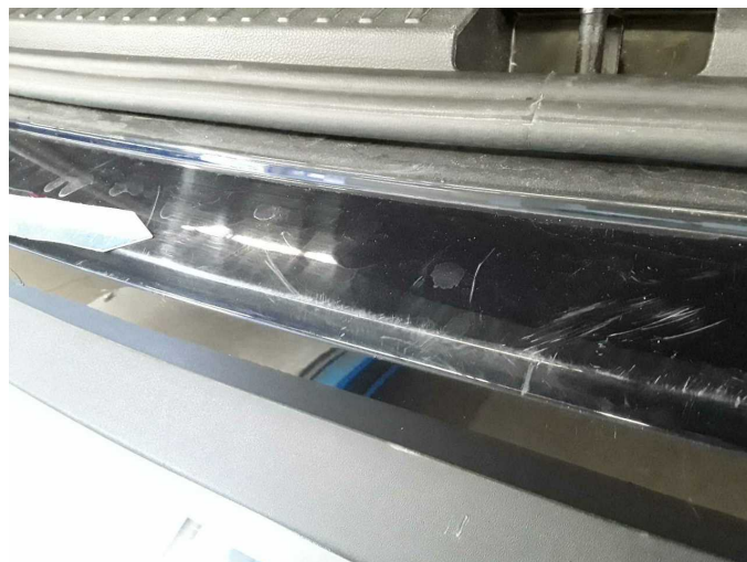
Damage 10: Rear bumper: Rear bumper - Scratched - Paint
