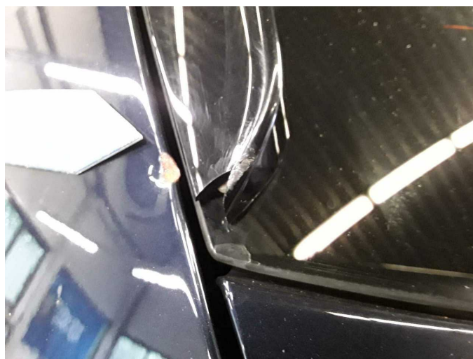
Damage 6: Boot lid / rear door: Trim - standard - lower - Damaged - Replace
