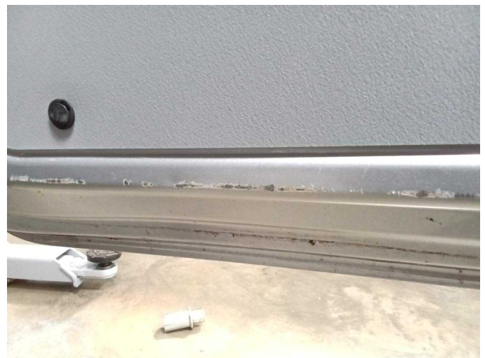
Damage 4: Boot lid / rear door: Rear door - right side - Scratched - Smart repair
