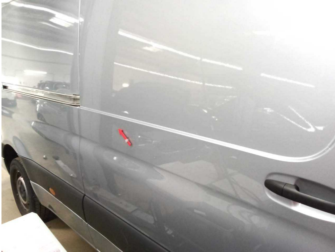
Damage 9: Sliding door, right: Sliding door - Dent / paintcoat damage - Repair and paint
