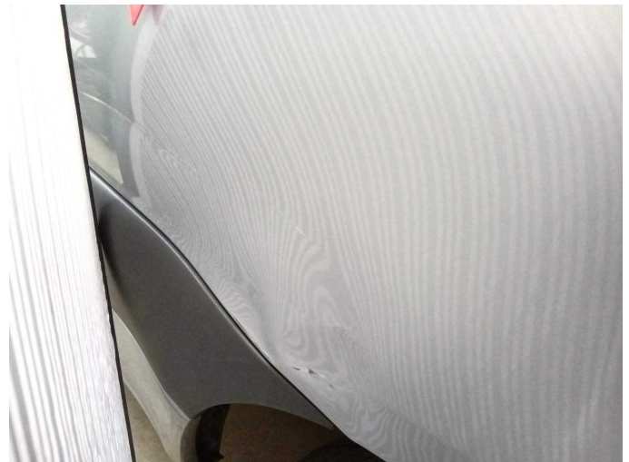
Damage 10: Side panel - rear left side: Side panel - Dent / paintcoat damage - Repair and paint
