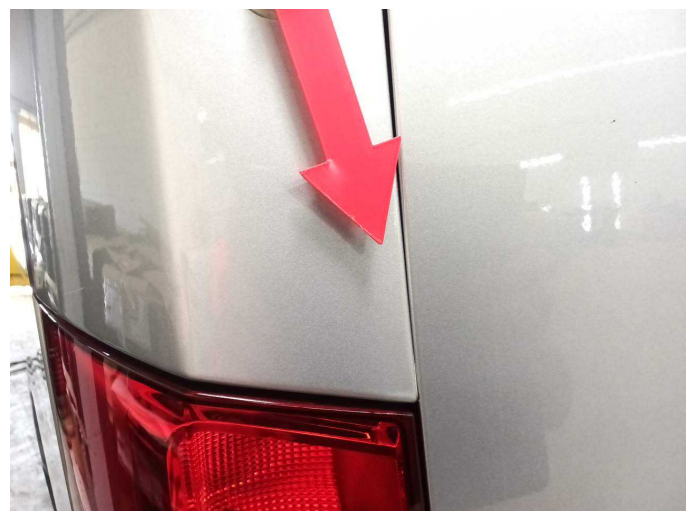
Damage 5: Boot lid / rear door: Rear door - left side - Malposition - Perform diagnosis
