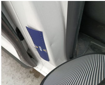
Rocker Panel Right // Smart Repair Medium-dent
