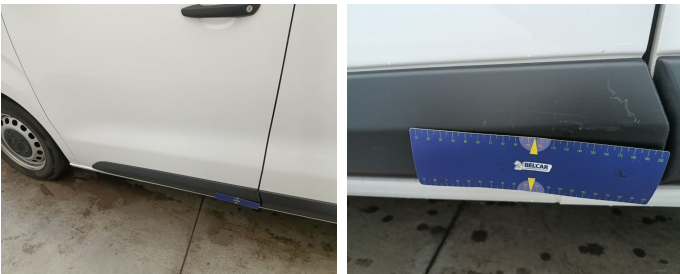
Door Front Left / Trim / Replace-scratch
