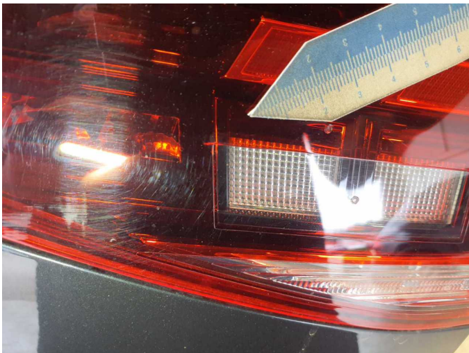
Damage 12: Tail light: Tail lamp - right side (innen) - Broken / torn - Replace
