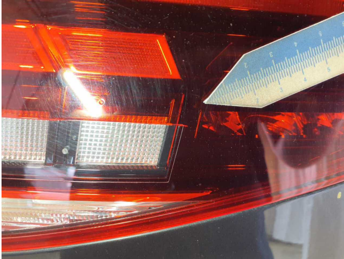
Damage 11: Tail light: Tail lamp - left side (innen) - Broken / torn - Replace
