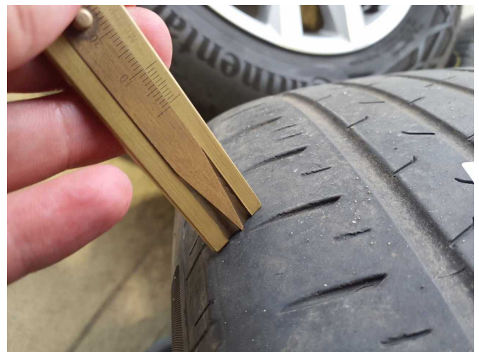
Damage 14: 2nd wheel set: Tyres - complete set - Worn - Replace
