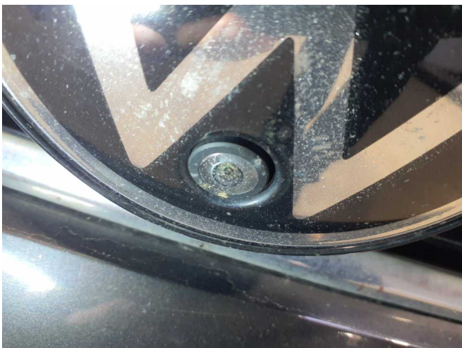
Damage 15: Electronic systems: Front camera - Stone chips - Replace
