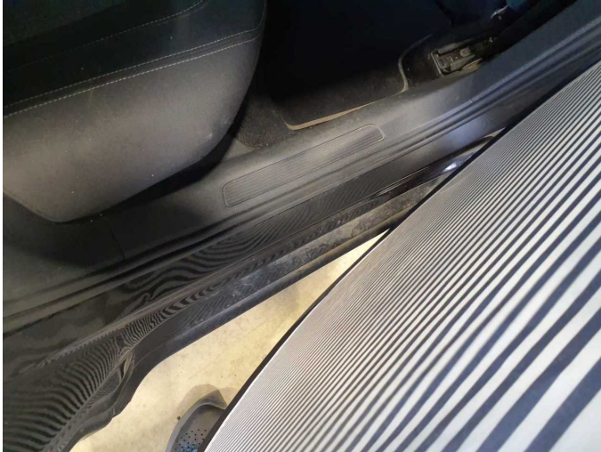
Damage 7: Side panel - rear right side: Sill - dent(s) - Smooth repair work
