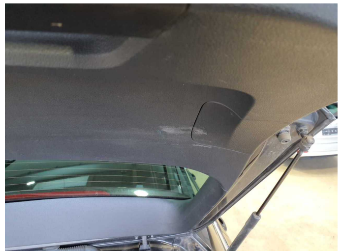
Wear and tear 8: Trim / covers: Boot lid - interior trim - Scratch(es) - No deduction
