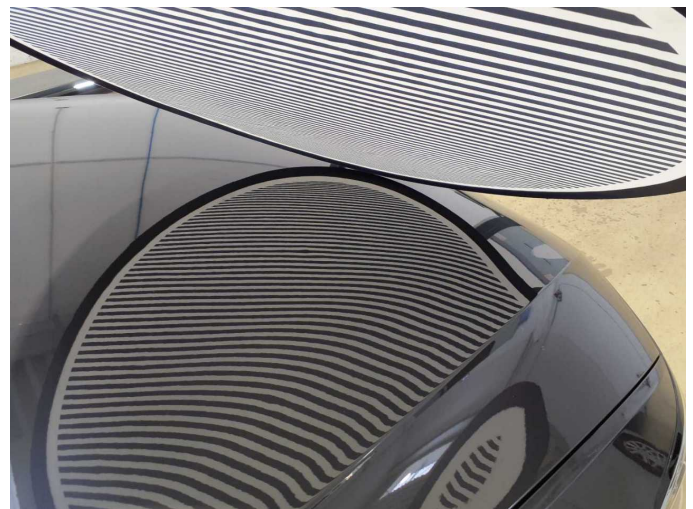
Damage 16: Body: Body (Korrosion an Dach & Motorhaube) - Damage by hail - Repair and paint
