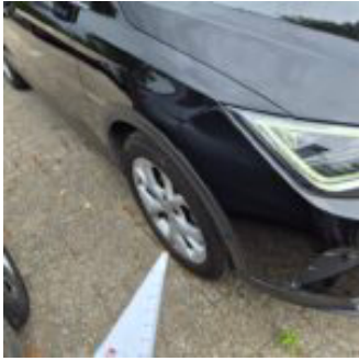
Damage Part Alloy - Right Front
