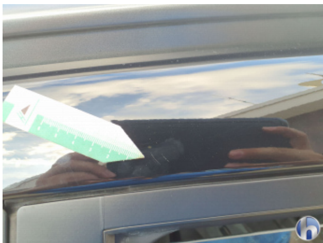
3. Dach Kratzer - Smart Repair
