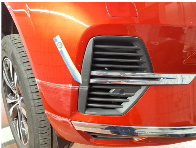
Damage 2: Front bumper: Cover bumper - front (Rechts Plastik) - Scratched - Replace
