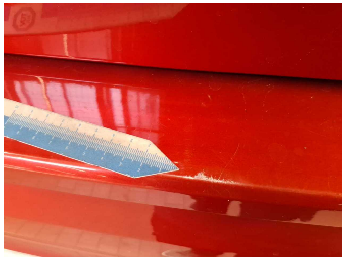
Damage 6: Rear bumper: Rear bumper - Scratch(es) - Paint
