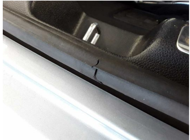
Damage #3: Boot lid / rear door: Seal - Porous / cracked - Replace
