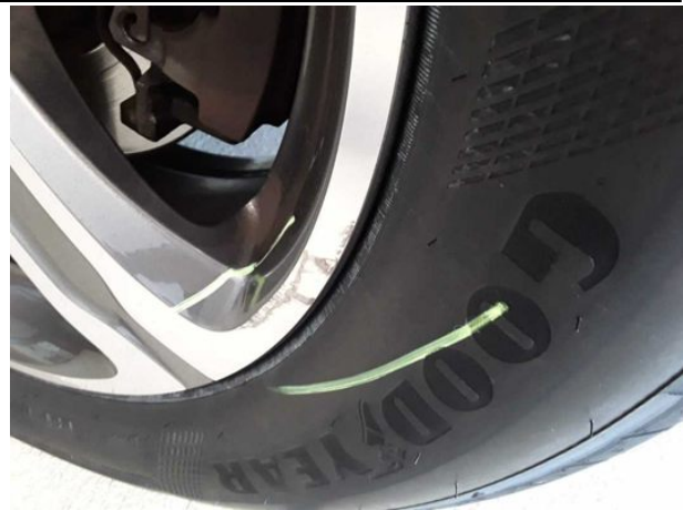
Damage #7: Wheel / tyres: Alloy rim - rear left side - Scratched - Loss in value
