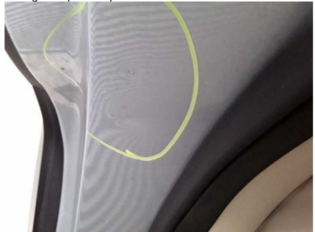
Damage #12: Side panel - rear right side: Sill - Dent / paintcoat damage - Repair and paint
