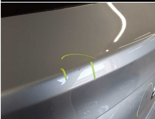
Damage #9: Boot lid / rear door: Boot lid - Dent / paintcoat damage - Smart repair
