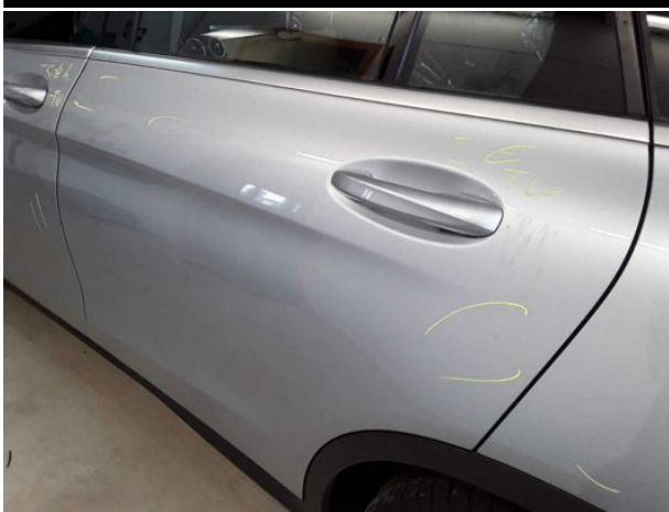
Damage #15: Door - rear left side: Door - Scratched - Repair and paint
