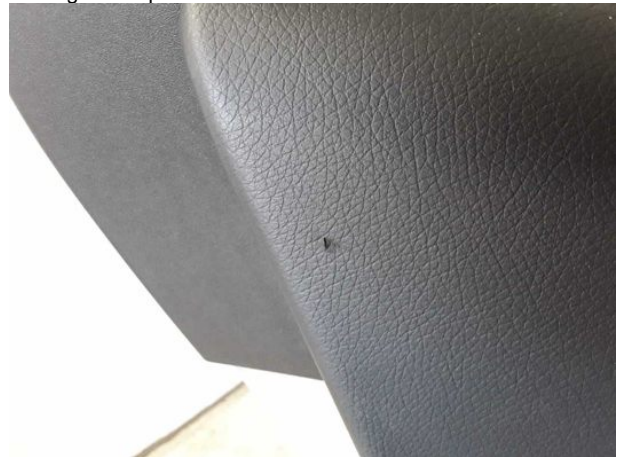
Damage #10: Trim / covers: Door trim - rear left side - Damaged - Replace
