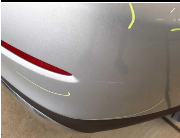
Damage #13: Rear bumper: Rear bumper - Scratch(es) - Repair and paint
