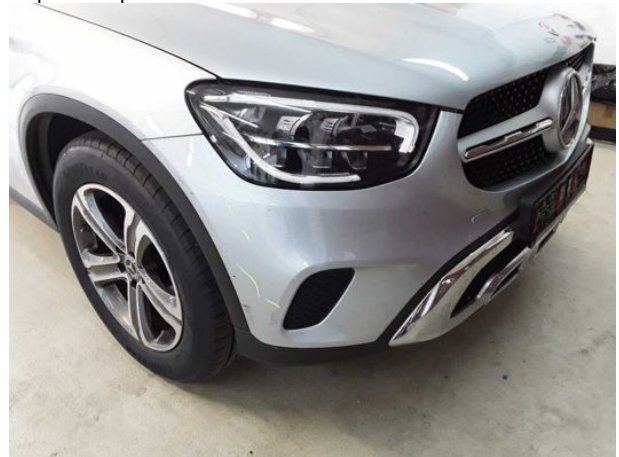
Damage #14: Front bumper: Front bumper - Scratched - Rep... and paint
