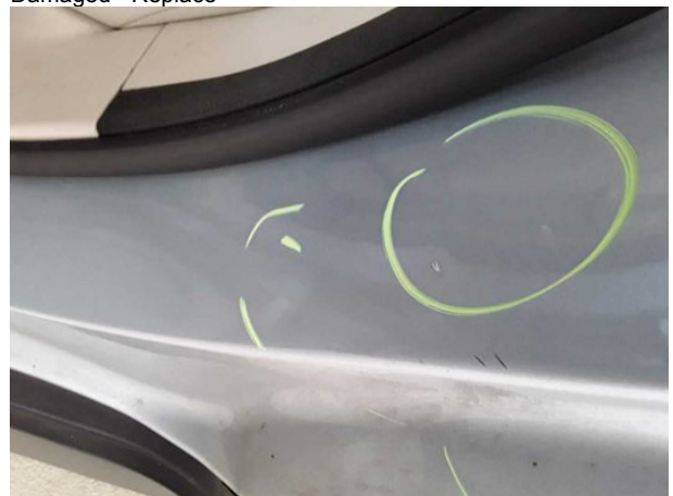
Damage #11: Side panel - rear left side: Sill - Dent / paintcoat damage - Smart repair
