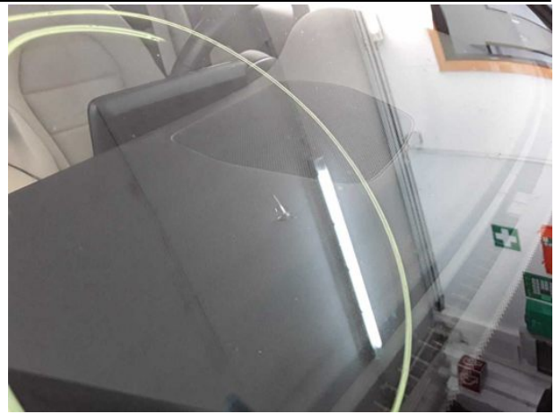
Damage #17: Vehicle glazing: Windscreen (Rissbildung) - Replace
