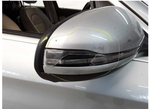
Damage #5: Indicator - front: Mirror - right side - Damaged - Replace
