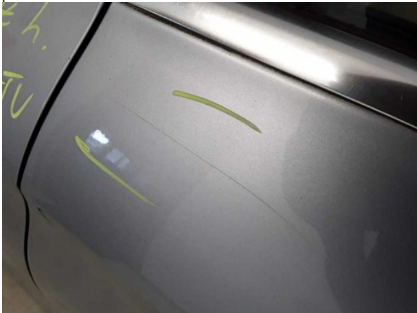
Damage #15: Door - rear left side: Door - Scratched - Repair and paint
