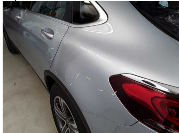
Damage #16: Side panel - rear left side: Side panel - Scratch... - Repair and paint
