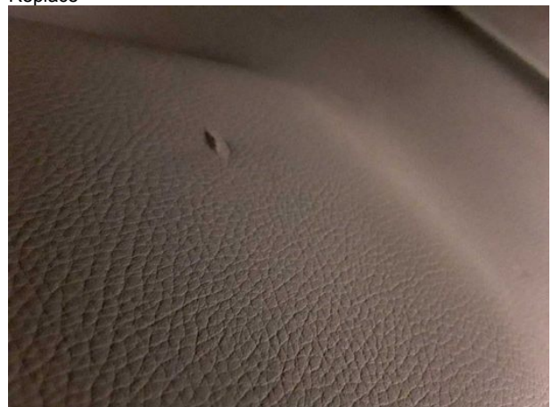
Damage #6: Seat - front: Seat base trim - left side - Damaged - Replace
