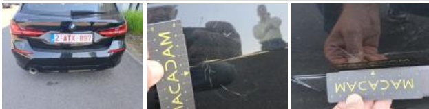
Step R, Scratch(es), Repair and paint (complete)
