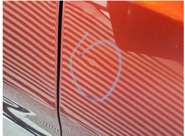
Damage #1: Mudguard - right side: Mudguard - right side - Dent / paintcoat damage - Smart repair
