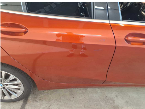
Damage #3: Door - rear right side: Door - Scratched - Repair and paint
