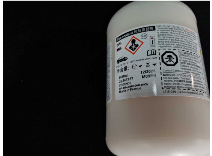
Damage 1: Equipment: Tirefit filler - Expired - Replace
