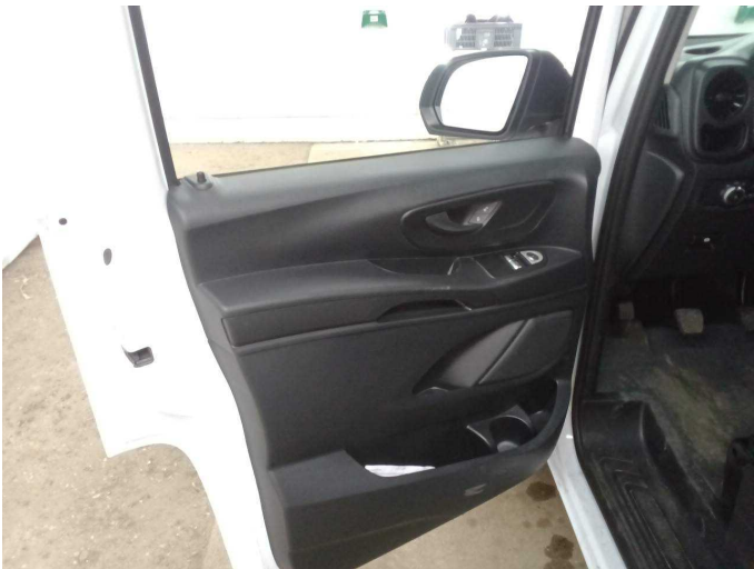
Damage 1: Trim / covers: Door trim - front left side - Scratch(es) - Loss in value
