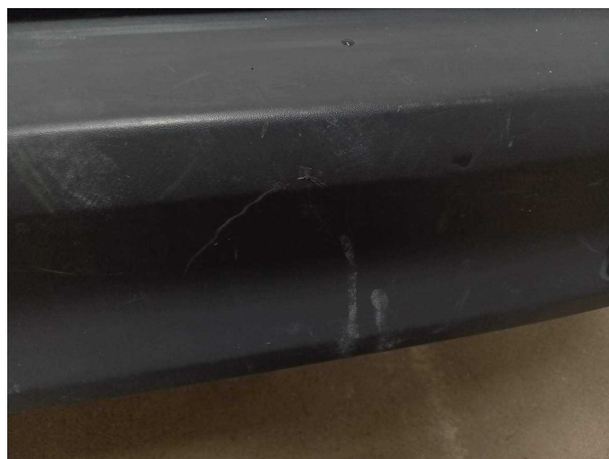
Damage 2: Rear bumper: Rear bumper - Scratch(es) - Replace
