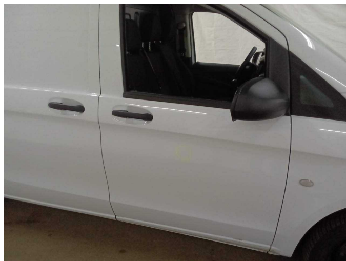
Wear and tear 1: Door - front right side: Door - dent(s) - No deduction
