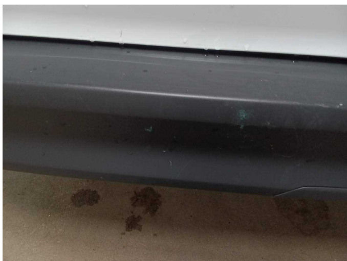
Damage 2: Rear bumper: Rear bumper - Scratch(es) - Replace
