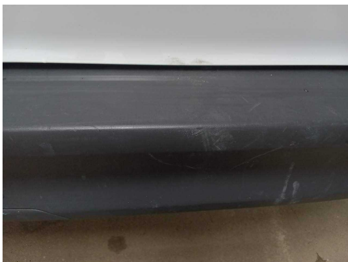
Damage 2: Rear bumper: Rear bumper - Scratch(es) - Replace
