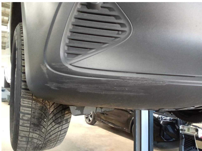
Damage 3: Front bumper: Front bumper - Scratch(es) - Replace
