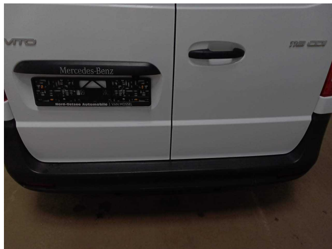
Damage 2: Rear bumper: Rear bumper - Scratch(es) - Replace
