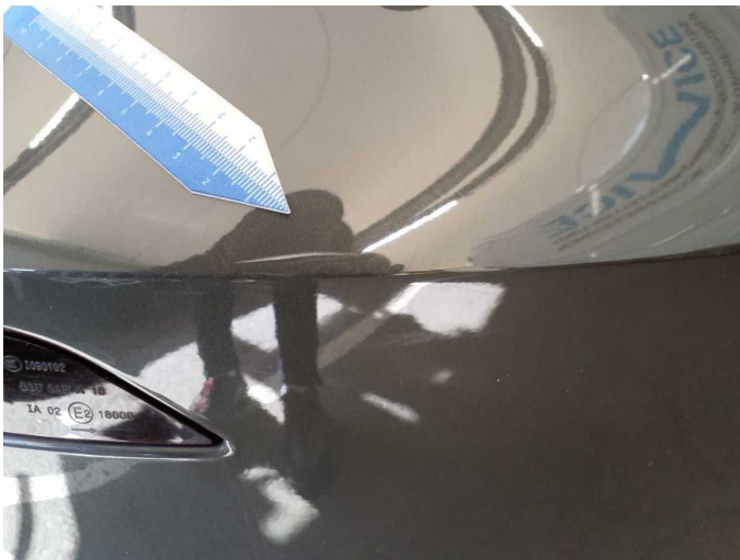
Damage 6: Rear bumper: Rear bumper - Scratch(es) - Paint
