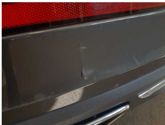
Damage 6: Rear bumper: Rear bumper - Scratch(es) - Paint
