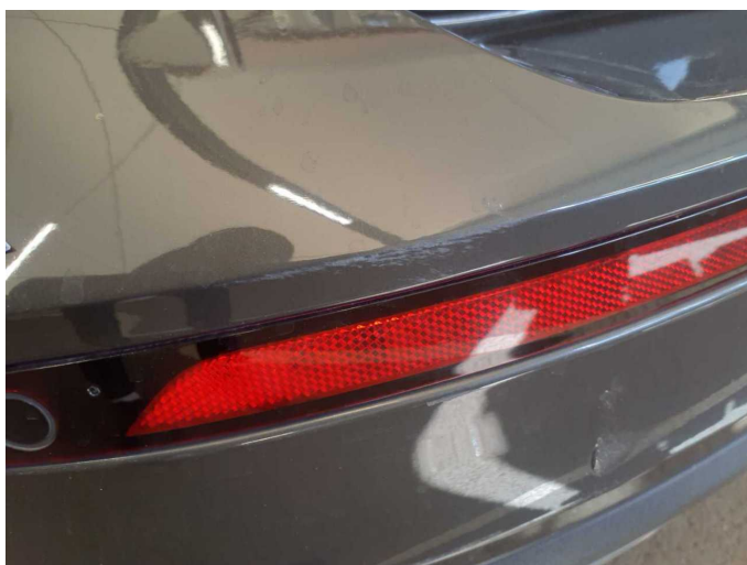
Damage 6: Rear bumper: Rear bumper - Scratch(es) - Paint
