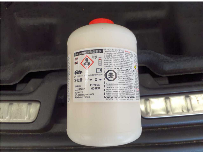
Damage 1: Equipment: Tirefit filler - Expired - Replace
