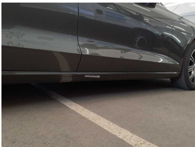
Damage 3: Sill - right side: Trim - Scratch(es) - Smart repair
