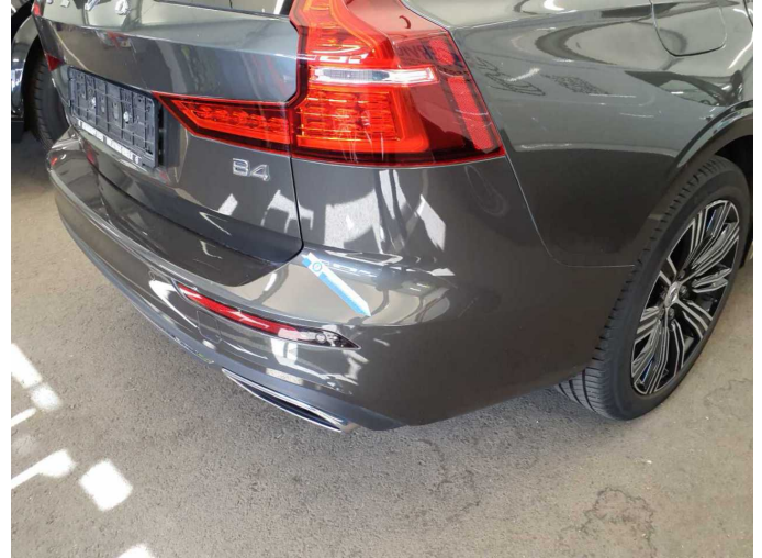
Damage 6: Rear bumper: Rear bumper - Scratch(es) - Paint
