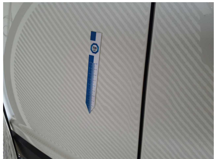
Damage 7: Boot lid / rear door: Rear door - left side - Deformed - Repair and paint
