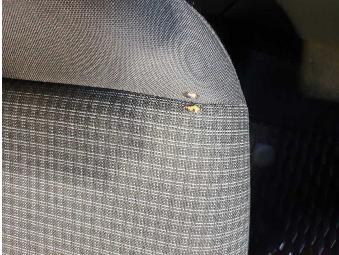
Damage 5: Seat - front: Seat cover - right side - Holes - Replace
