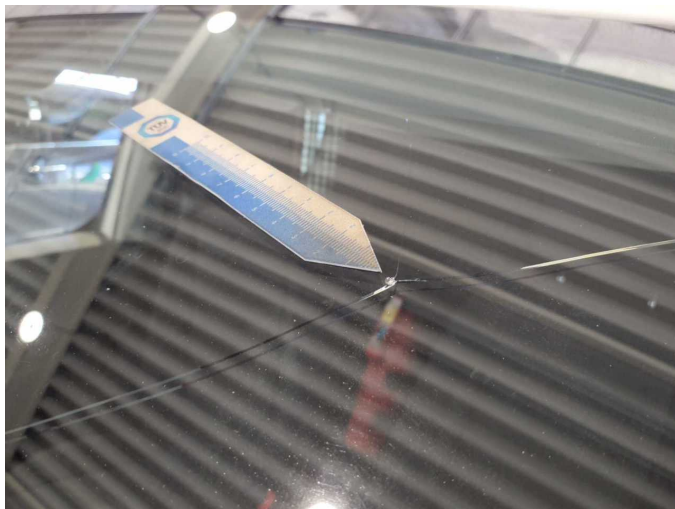
Damage 8: Vehicle glazing: Windscreen - Broken / torn - Replace
