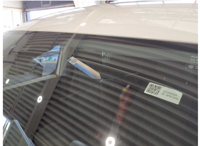
Damage 8: Vehicle glazing: Windscreen - Broken / torn - Replace
