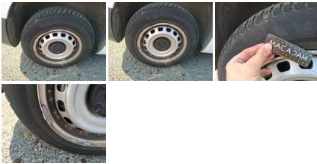
Steel rim RR, Deformed / Strained, Replace
