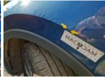
Wing FL, Dent(s) and scratch(es), Repair and paint (complete)
