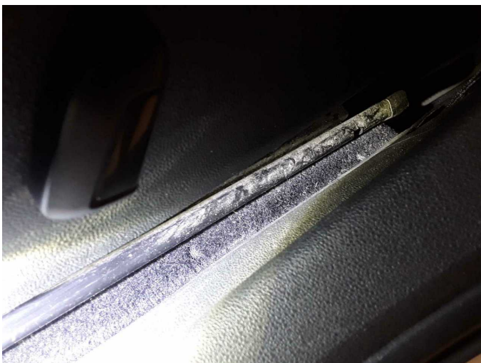
Damage 7: Trim / covers: Floor covering - front left side - Burn hole (cigarettes) - Loss in value
