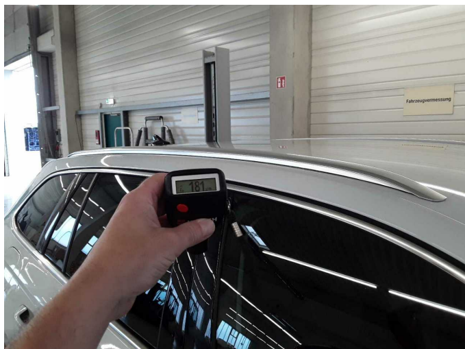
Roof rail - right side: 181 \mu\text{m}
