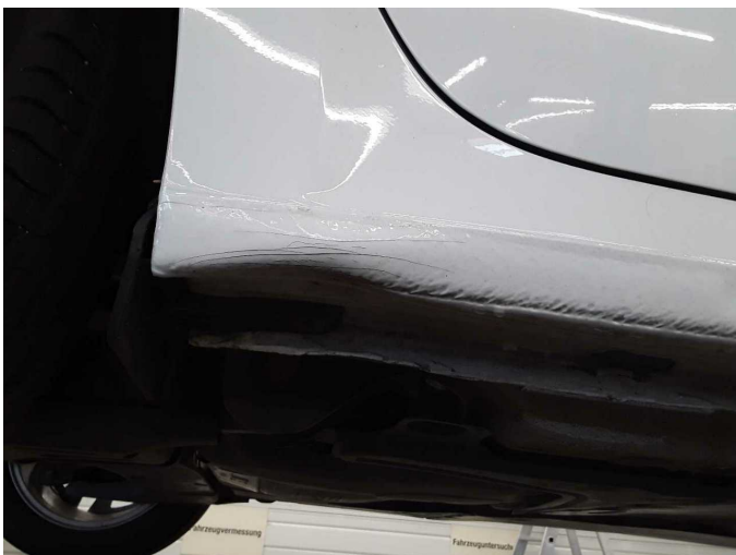
Damage 10: Sill - right side: Sill - Deformed - Repair and paint
