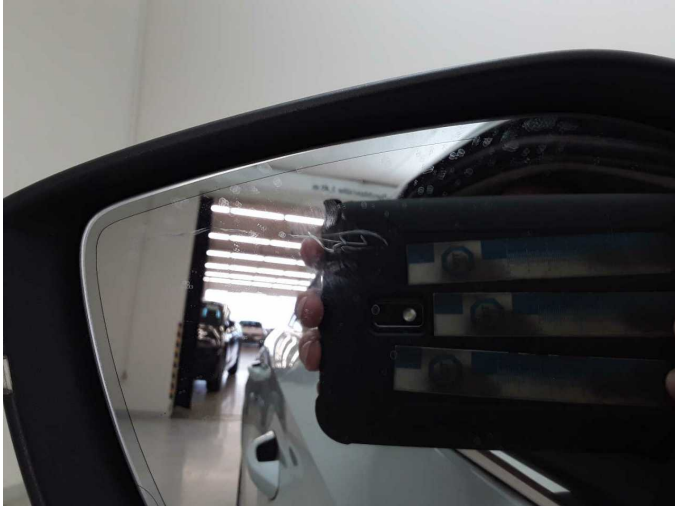
Damage 8: Wing mirror - left side: Mirror glass - Scratch(es) - Replace
