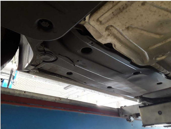
Damage 3: Body: Underbody panelling (rechts) - Broken / torn - Replace
