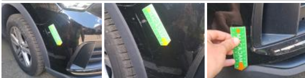
Bumper moulding F, Deformed / Strained, Replace
