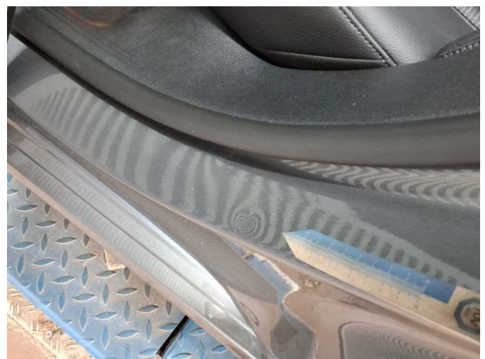
Damage 3: Side panel - rear left side: Sill - dent(s) - Smart repair
