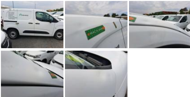
Sliding door R, Hail damage, Repair and paint (complete)
